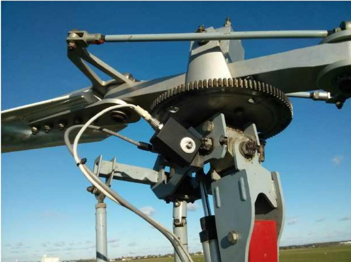
**Fig 2.3. Sensors Mounted On Rotor Head**
